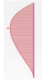
Bending moment diagram M_x = 3.27 \text{ tons}\cdot\text{m}
